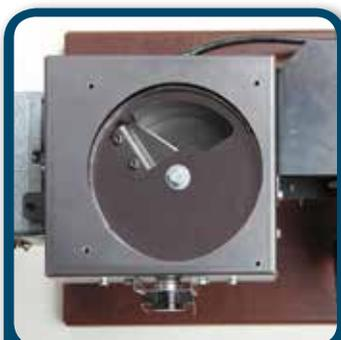
*NEW HRD feed system features case hardened cutting blade to cut through the toughest pellets!*
